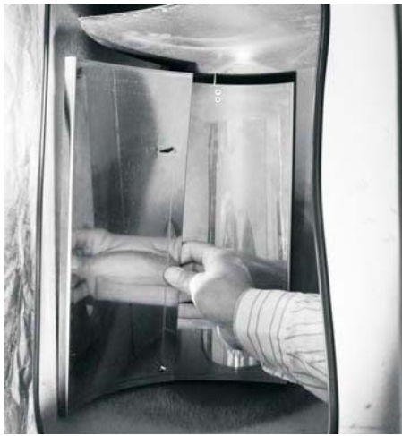
FIGURE 20: Place Part B over stud bolts in Part A.
