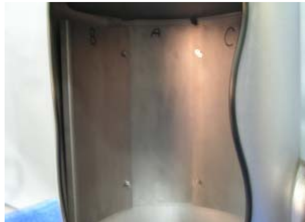
FIGURE 23: Inspect with light to make sure Part A, B, and C are pushed outward against drum.
