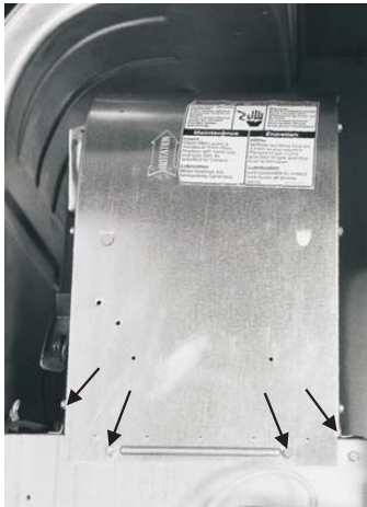
FIGURE 32: Remove Blower Assembly Mounting Screws (4). Unplug blower motor from control box. Remove wire clamp. Remove blower assembly.
