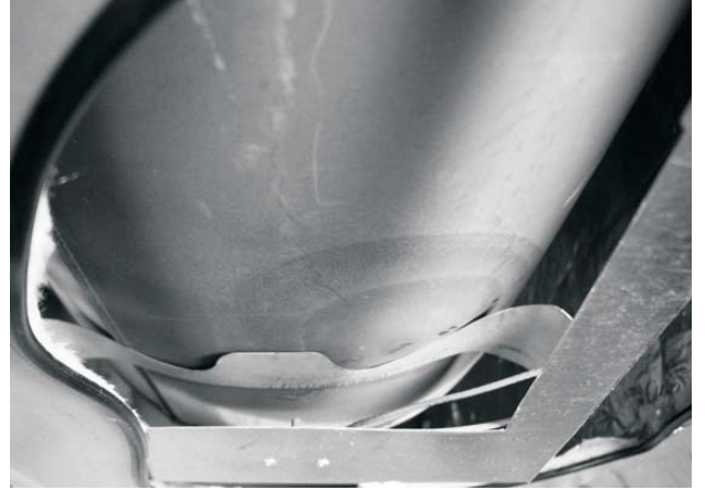
FIGURE 40: Outer plate should compress against side casing foil (Cut-away view).
